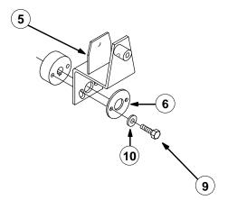
Mount the shock absorber to the new propel lever plate (5) with set aside hardware. (Refer to FIG. 2, p.9)
