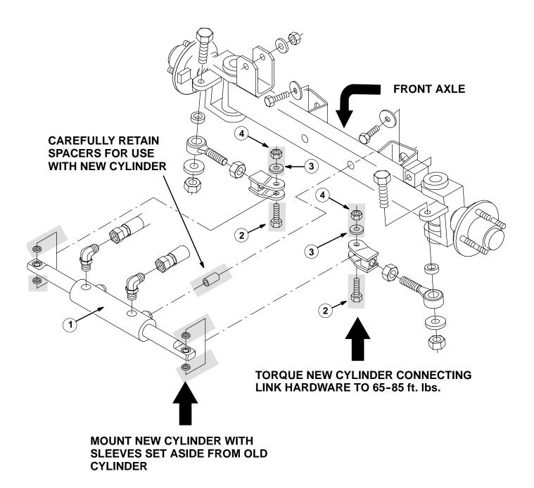
FIG. 1 - NEW HYDRAULIC CYLINDER INSTALLATION
