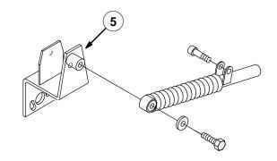
8. Mount the rod end and bracket assembly with new spacers (8), inside the new propel lever plate (5), with new socket screw (7) and nut (11). Torque the socket screw (7) to 19–25 ft lbs. (Refer to FIG. 2, p.9)
