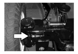
3. The wheel axle casting should NOT BE touching the stop bolt. There should be .030" clearance between the head of the stop bolt and the edge of the wheel axle casting.
